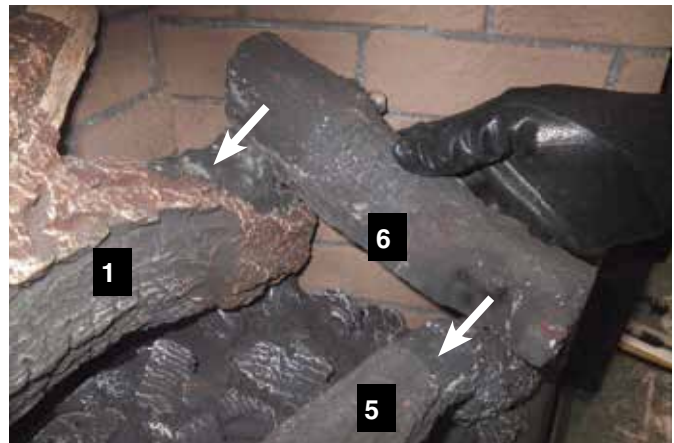
8. Line locator at top of Log 6 with provision on Log 1 - the locator at the bottom of Log 6 should line up with the provision on Log 5.
